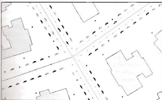
Figure 1: To represent a two-way traffic street, the centerline is duplicated, and each copy is employed for representing one direction. Parking places are built parallel to the street, with a distance of 4 meter between the places. Destinations are represented by the set of points constructed in front of the entrance to the building (red triangles in the map).
